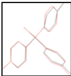
Fig. 2. Superimposed wireframe drawing of the two molecules of \text{SeP(4-FC}_6\text{H}_4)_3 in the asymmetric unit. H atoms have been omitted for clarity. The molecule containing P2 is indicated in red.
